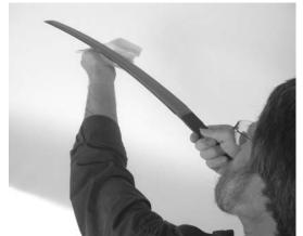
Slide the habaki onto the tang the tsuba and washers in their original the handle vertical and lower the nakago into the handle. Maintain the sword in position and tap on the bottom of the the heal of your free hand. A few taps sufficient to firmly seat the nakago in Replace the mekugi through the hole in
